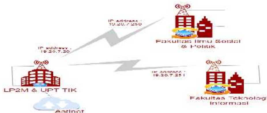
Gambar 2. Topologi Jaringan Point to Multipoint USN kolaka [7]
